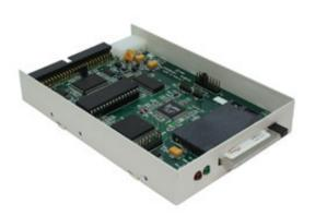
Peripheral Vision Tech LTD (PV) (Reading UK), have developed a Solid State Disk drive, Magneto Optic (MO) and Tape drive with emulation capability aimed at ageing drives in the DMS10 and other legacy Telco systems. This is a SCSI tape or SCSI disk drive with no moving parts in a 3.5" or 5.25" form factor.
