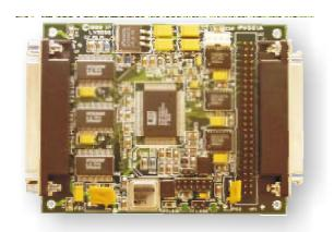
The LVD-2-SE will convert single-ended peripherals to wide Low Voltage Differential (LVD). This prevents the Ultra2 SCSI LVD bus from defaulting to the Single Ended bus, with the resultant loss in performance.
